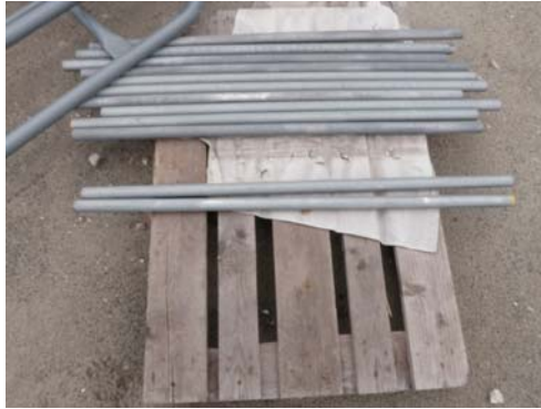
Pic. 1.2 Galvanized threaded anchor bolt
